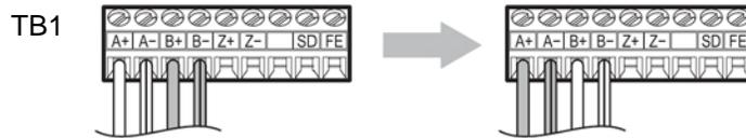
**Figure 11: A Channel and B Channel Wire Switching**
