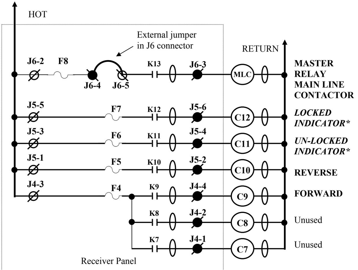
*\*NOTE: K12 remains closed if the unit is locked and the receiver is turned OFF by the transmitter. K11 will open if the unit is unlocked and the unit is turned OFF by the transmitter.*
