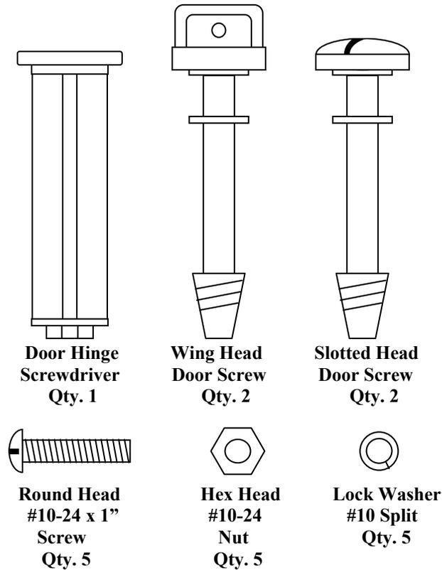
**Figure 4-1A. Installation Hardware.**
