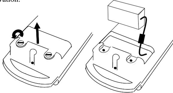
Figure 4-3. *telePendant* Battery Replacement.
