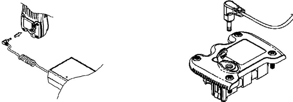
**Figure 3: Plugging in the Charging Cable**
