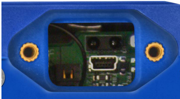
Figure 8: USB mini-B receptacle as viewed through USB/IR port
