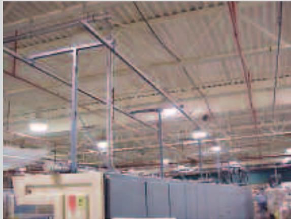
It consists of a special filter-equipped vacuum, a festoon system that supports the vacuum hose and a T-bracket that holds the festoon system in place. The festoon is situated on both sides of the sorting machines and each vacuum system services two machines. This configuration allows the user to clean the entire length of the sorting machine without dragging the hose on the floor.
